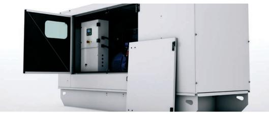
Side hinged doors, on each side of the enclosure, provide ample access to all necessary components during installation and servicing. Lift-off hinges enable the doors to be removed at an angle of 90°, facilitating easy servicing in confined installation spaces.
