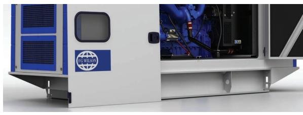
Side hinged doors, on each side of the enclosure, provide ample access to all necessary components during installation and servicing. Lift-off hinges allow doors to be removed, even at an angle of 45°, facilitating servicing in the most confined installation spaces.
