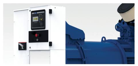
The common control panel tower mounted on the end of the set, is close coupled with set mounted breakers (up to 1600A) utilising high performance, durable copper braids. The tower has a split box design providing total access to all components and wiring.
